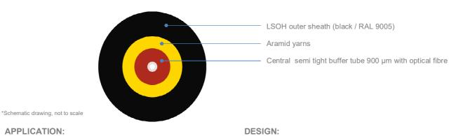
For installation on poles Fully dielectric Aerial cable with aramid reinforcement Semi tight buffer with 1 optical fibre (0.9mm) Module with 2 optical fibres (option) Aramid yarns LSOH outer sheath
