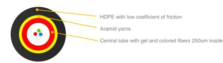
\*Schematic drawing, not in scale
